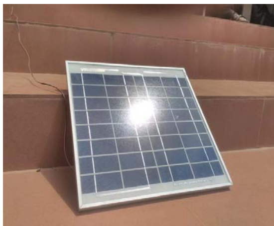
Figure 6.1: Solar panel of 60W
